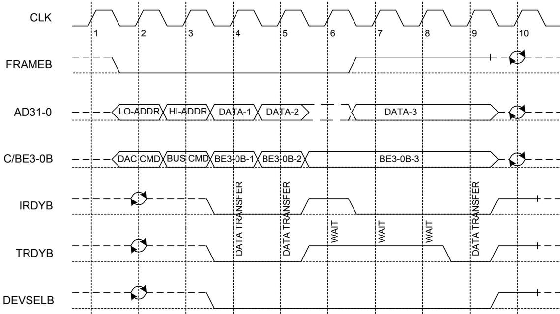
**Memory Write above 4GB (DAC, 64-bit address, 32-bit data; 32-bit slot)**
