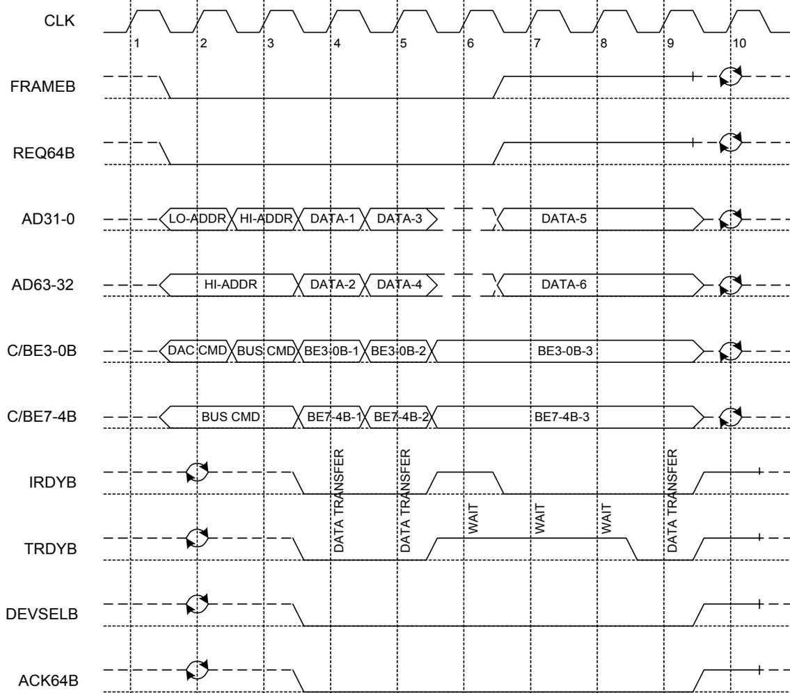
**Memory Write above 4GB (DAC, 64-bit address, 64-bit data transfer granted; 64-bit slot)**
