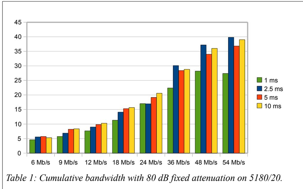
Table 1: Cumulative bandwidth with 80 dB fixed attenuation on 5180/20.
