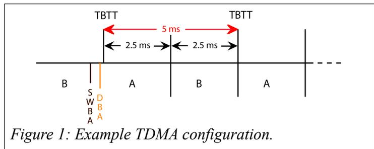
Figure 1: Example TDMA configuration.
