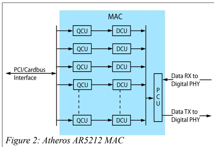
scheduling algorithm where frames are dispatched according to the beacon timer for sending beacon frames. By applying this frame scheduling algorithm to the normal data frames the hardware can be used to schedule data frames according to the beacon schedule.
