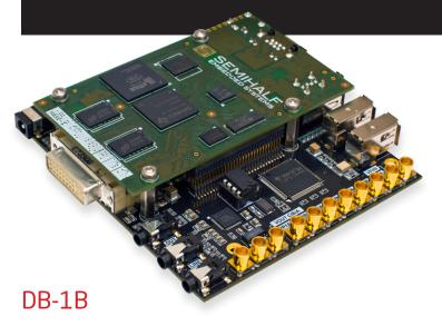
DB-1B complements and extends the main HASE-1 video processing module hosting the Texas Instruments Digital Multimedia system-on-chip, and allows for rich connectivity options to be used with the main processing module.
