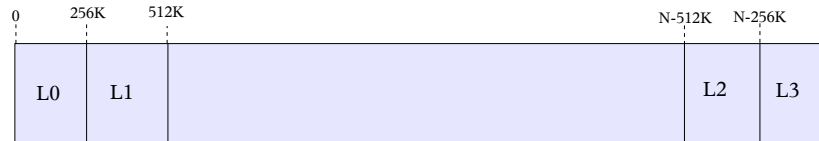
Illustration 2 Vdev Label layout on a block device of size N
