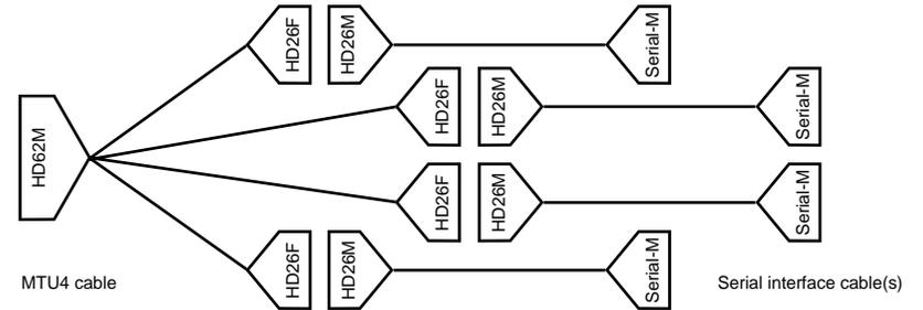
The available serial interface cables are as shown for the FarSync T2Ue on page 2.
