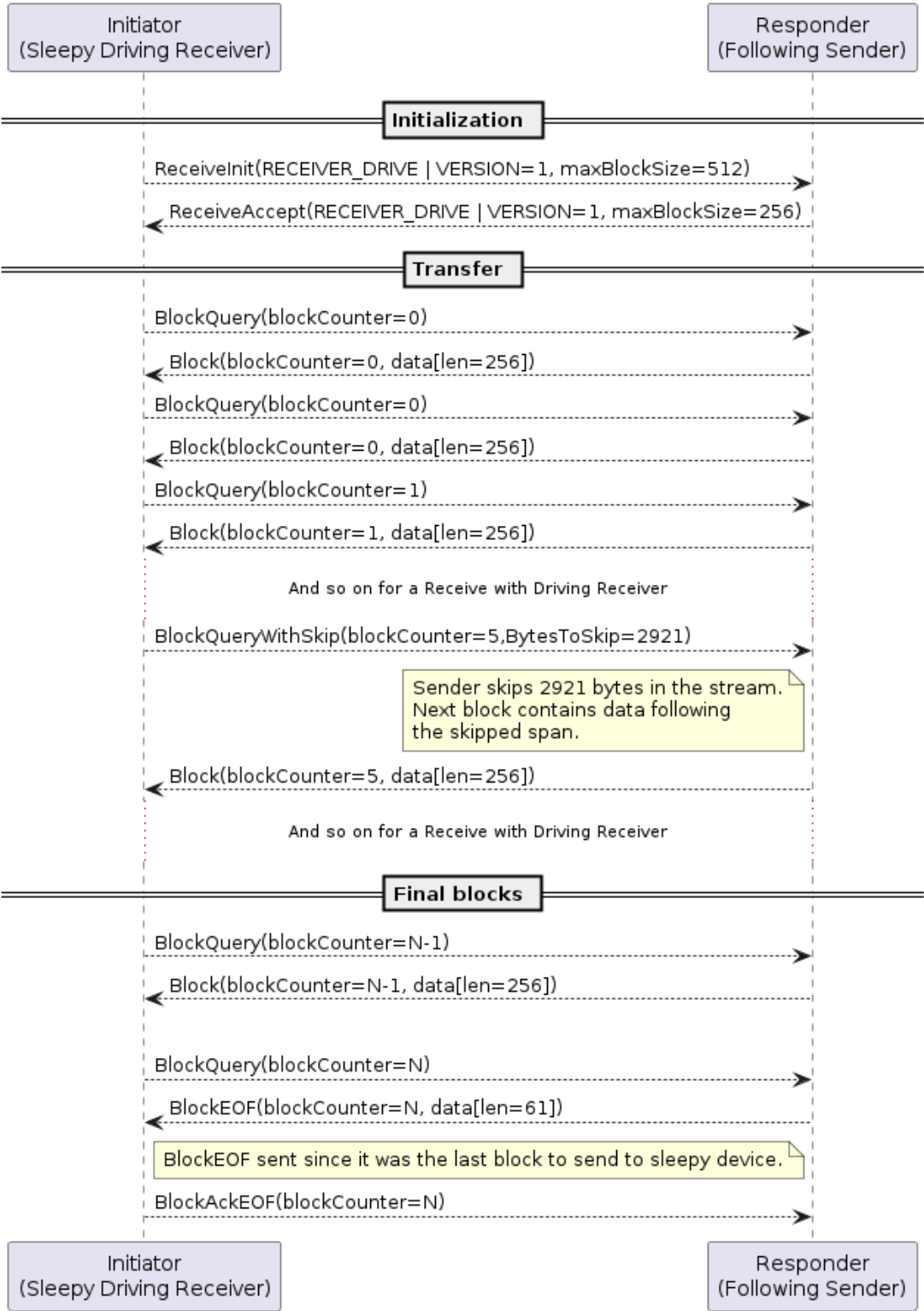
Figure 90. Synchronous file receiving by device acting as driving Receiver, including BlockQueryWithSkip
