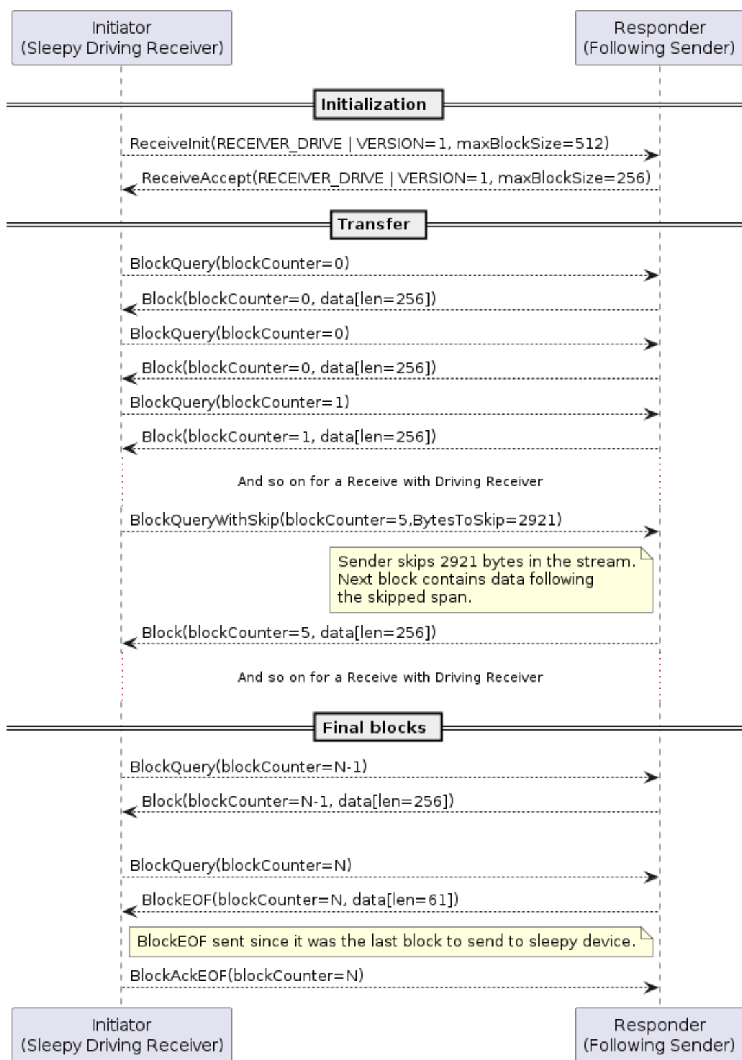
Figure 95. Synchronous file receiving by device acting as driving Receiver, including BlockQueryWithSkip
