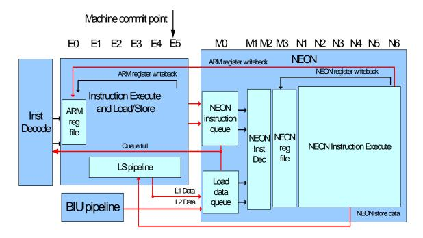
The NEON unit is decoupled from the main ARM integer pipeline by the NEON instruction queue (NIQ). The ARM Instruction Execute Unit can issue up to two valid instructions to the NEON unit each clock cycle. NEON has 128-bit wide load and store paths to the Level-1 and Level-2 cache, and supports streaming from both.
