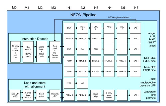
VFPv3 Floating Point Specification targeted for medium performance IEEE 754 compliant floating point support. VFPLite is used to provide backwards compatibility with existing ARM floating point code and to provide IEEE 754 compliant single and double precision arithmetic. The "Lite" refers to area and performance, not functionality.
