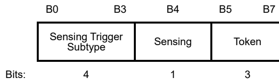
Figure 9-103a—Trigger Dependent Common Info field format of the Sensing Polling, SR2SI Sounding, Sensing Reporting, and Sensing Threshold-Based Reporting Trigger frames
